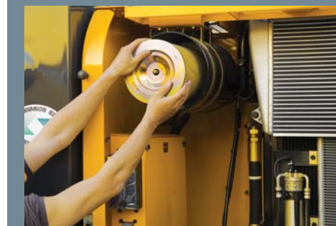
Easy to Change Air Cleaner Assembly Air cleaner is centralized in one or the same compartment for easy service.
